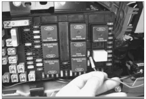
**6.** Remove the OBD II interface cable from the vehicle.
