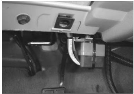
Figure 18 Brake Position Sensor location under dash
