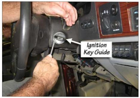
Figure 20 Remove Plastic Ignition Key Guide
