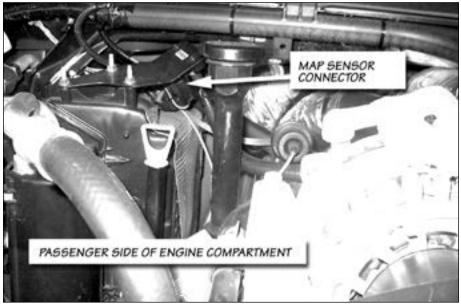
Figure 8: MAP sensor harness routing
