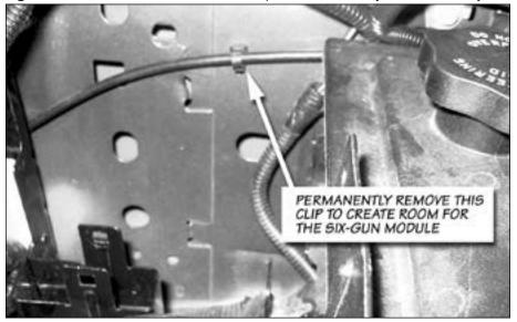
Figure 12: Removal of hood latch cable clip (2003-04 model year vehicles only)
