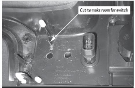
fully rotated counterclockwise. Secure the switch(s) with the internal tooth washer(s) and nut(s). Snug the nut(s). Be careful not to over-torque the nut(s) and damage the threads.
