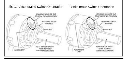
Figure 28: Finished installation of the Six-Gun/EconoMind/Brake switchs on 2003-04 vehicle
